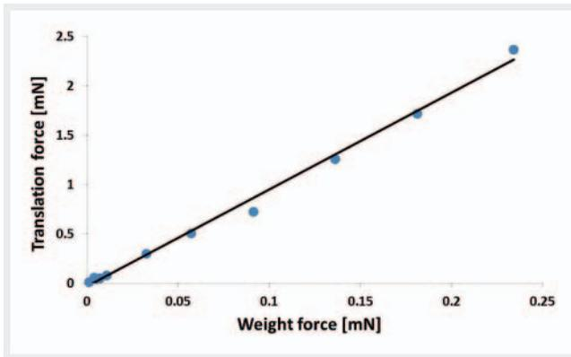
► **Fig. 3** Translation force as a function of the weight force of the 10 steel plates in a 3 T MRI (gradient of the straight lines: 9.62; coefficient of determination R<sup>2</sup>: 0.99).
