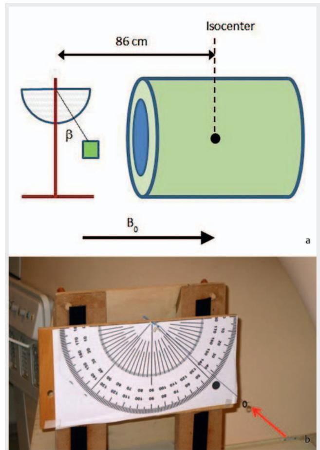
► **Fig. 1** a Schematic illustration of the translational force apparatus [10]. The deflection angle β is measured to the direction of the magnetic field B<sub>0</sub>. b Translational force apparatus (wooden) with paper protractor and the suture mounting made of plastic. The steel plate (marked by a red arrow) and the additional weight (rubber ring) fixed on a suture.
