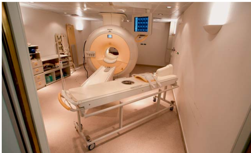
Fig. 1 HIFU treatment unit: patient table with integrated ultrasound transducer in front with the MRI scanner in the background.
