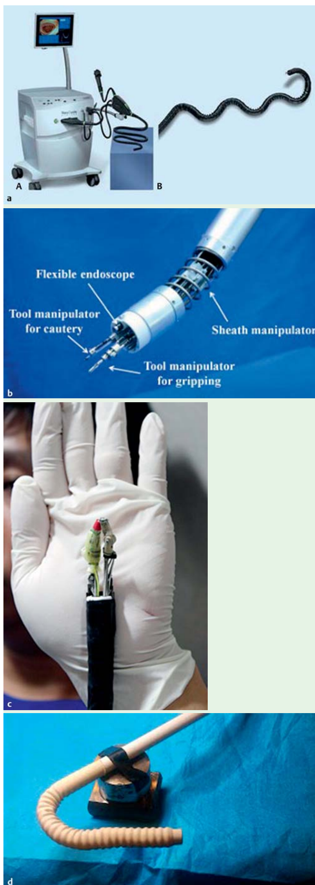
Fig. 2 Robotic interface platforms. a NeoGuide; b Master-slave system (IRCAD); c MASTER; d i-Snake.
