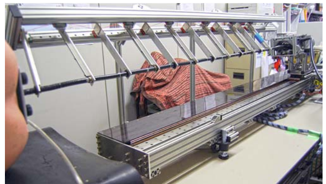
► Fig. 2 The slave unit of Endoscopic Operation Robot (EOR) ver. 3. to which the colonoscope (Olympus PCF-240; Tokyo, Japan) is attached.
