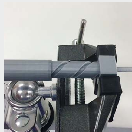
► Video 1 Prototype demonstrating the conversion of axial force to axial movement combined with rotation of the needle tip. (representative still image of the video).
