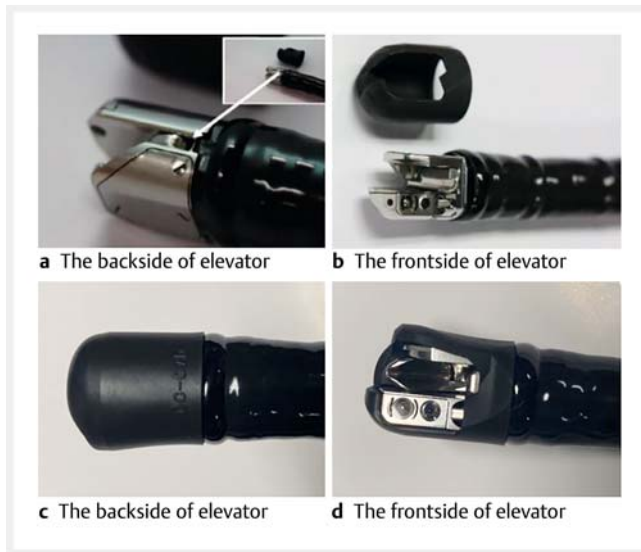
► Fig. 1 A newly designed duodenoscope with detachable distal cap (ED 580XT; Fujifilm, Tokyo, Japan). a,b The distal cap was detached before manual cleaning to allow the brush to access the back of the elevator (white arrow). c,d The distal cap was not detached before manual cleaning in order to imitate the conventional duodenoscope with a fixed distal cap.
