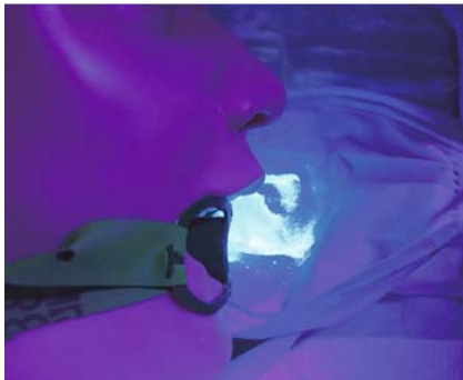
► Fig. 4 Excessive amounts of dye were found inside the modified surgical mask when worn by the “patient.”
