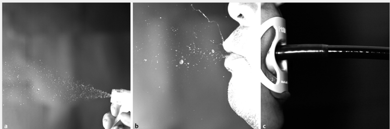
► Fig. 1 Photographic analysis of droplets using a high speed camera showing: a microscopic droplet release through a spray bottle; b droplet ejection from a normal coughing model; c the results of filming around the entry point of the endoscope during a procedure.
