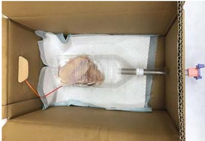
► **Fig. 1** Setting the skinned chicken meat with an electrode in a 2-L polyethylene terephthalate bottle.
