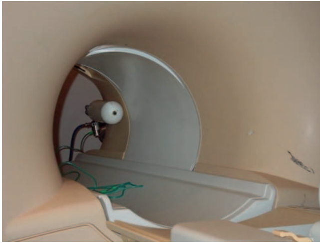
► Fig. 1 Photograph of an oxygen bottle in a 3 T whole-body MRI unit. A non-MR-safe oxygen bottle was carried into the MRI room and attracted by the strong magnetic field causing it to be catapulted into the MRI unit.
