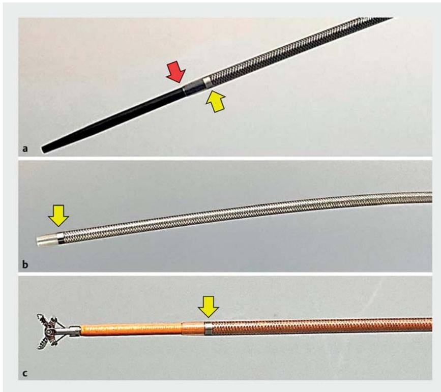
► **Fig. 3** Images of the novel device delivery system showing: **a** the tip of the system with no caliber difference between the inner catheter and outer sheath (red arrow), which has a radiopaque marker at its tip (yellow arrows); **b** the shape of the outer sheath after the inner catheter has been pulled out; **c** the biopsy forceps inserted into the outer sheath.
