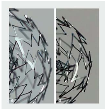
► Fig. 1 Cell width of the novel uncovered self-expandable metal stent (YABUSAME; Kaneka, Tokyo, Japan) is small compared with the conventional type, particularly in the part where bending force is applied. a YABUSAME stent. b Conventional uncovered self-expandable metal stent.
