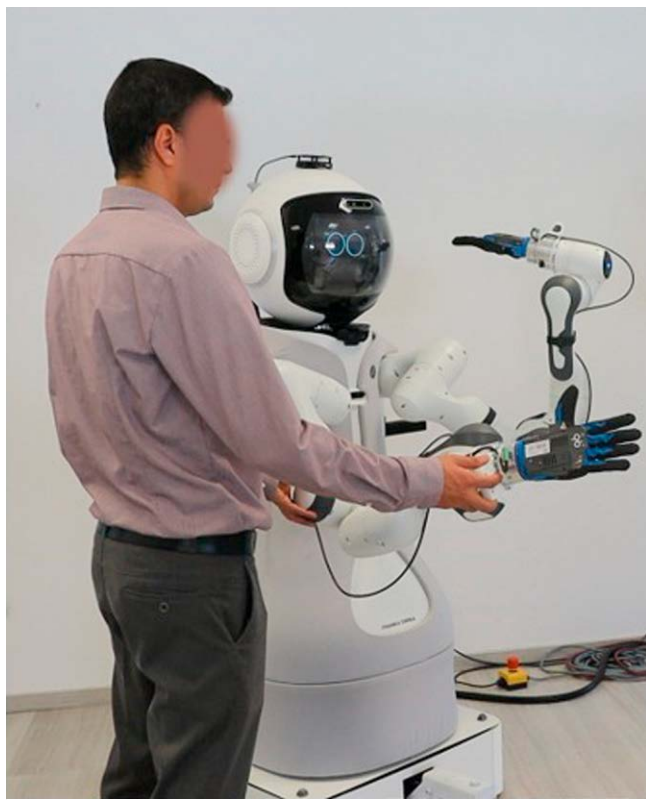
► Fig. 1 GARMi, A service robotic platform embedded with appropriate level of intelligence for daily living and healthcare applications.
