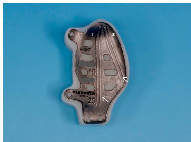
► Fig. 2 Patient-specific implant for reconstruction of the right orbita (KLS Martin Group, Tuttlingen, Germany) with several functionalizations. Arrows: trajectories for intraoperative navigation; + preventive design with caudally angulated dorsal support (inverted snow shovel); * reconstruction of the posterior medial bulge.
