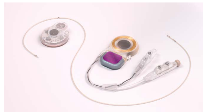
► Fig. 6 LP system components (laryngeal pacemaker development project of MED-EL company) consisting of a microelectrode for opening stimulation of the posterior crico-arytenoid muscle (PCA), the LP implant with inductive transmission coil, and connectors for 2 electrodes and the external LP processor with control unit and battery.
