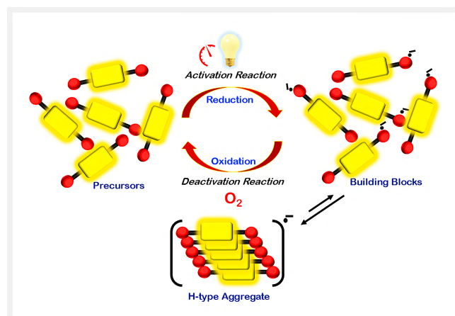
Scheme 2 Light-driven dissipative self-assembly of photo-reduced DIPFPDI .
