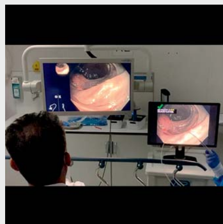
► Video 1 An example of our POLAR system. If the endoscopists detect a polyp, they take an image using narrow-band imaging. Subsequently, the system localizes the polyp, performs a quality check, and performs an optical diagnosis. In this video, the POLAR system predicts with high confidence that this is an adenoma (confidence level of 81%). Online content viewable at: https://doi.org/10.1055/a-2009-3990
