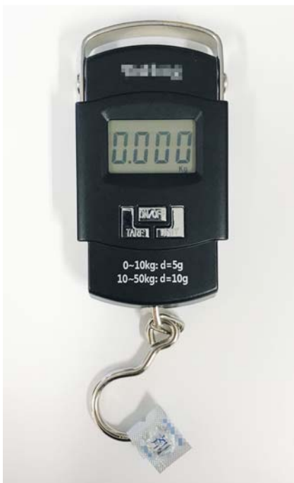
► Fig. 2 A PTP sheet was attached to the tip of the spring scale to evaluate the gripping force of various devices.
