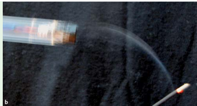
Fig. 3 Effect of the fan devices on the flow of smoke created with incense sticks: a blowing type; and b ventilation type.
