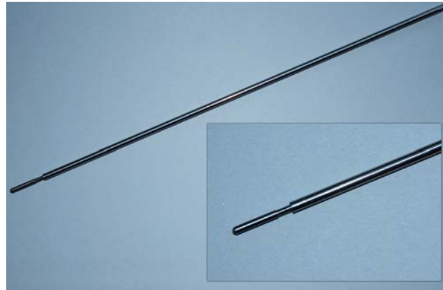
Fig. 2 The stainless steel probe (length 27 cm, diameter 3 mm) that is thinner at the tip (length 3 cm, diameter 2 mm).
