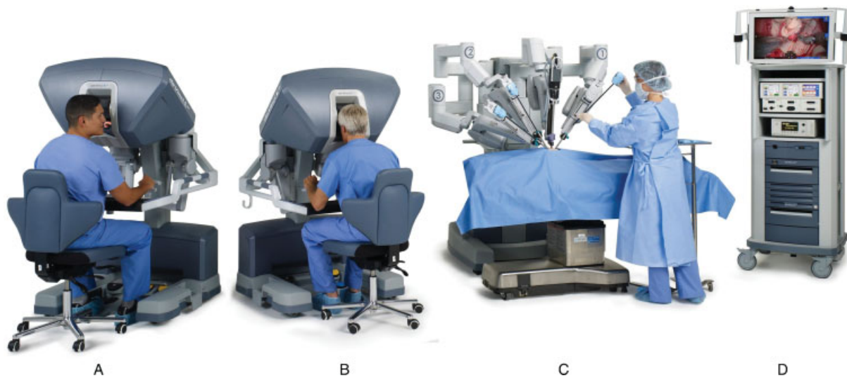
Figure 1 Current version of the da Vinci Si robotic surgical platform by Intuitive Surgical. (A) Surgeon's console. (B) Optional second surgeon's console. (C) Patient-side cart with four robotic arms and exchangeable instruments. (D) Laparoscopic tower with main computer. (Copyright Intuitive Surgical, Inc. Reproduced with permission.)
