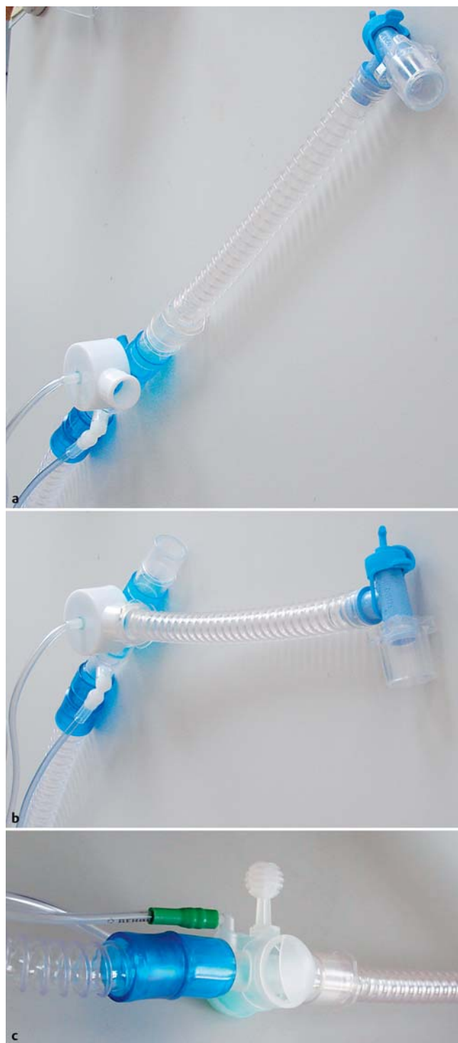
Fig. 1 a Breathing tube with active expiration valve (white) and extension tube. b Misconnection by combining the extension tube directly to the expiration valve, thereby interrupting the ventilation. c A technical solution preventing misconnection of the breathing tube.
