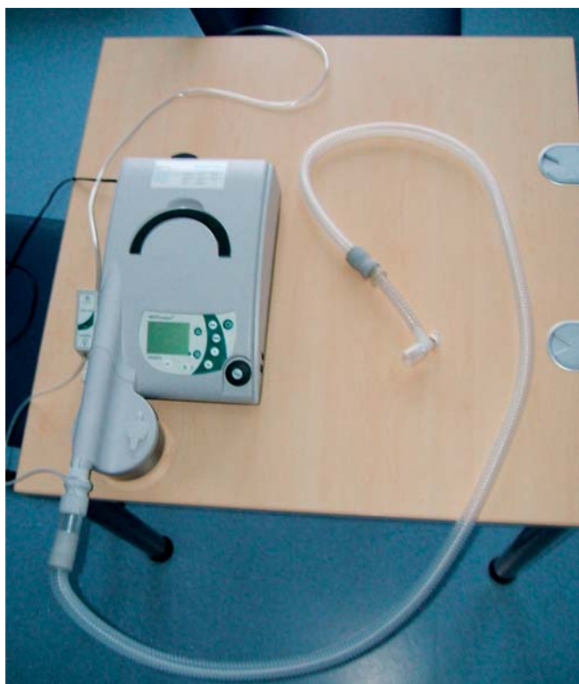
Fig. 2 Misconnection of a ventilator designed for non-invasive ventilation to the extension of an endotracheal tube. The ventilator tube has no expiration valve, so that rebreathing of CO 2 occurs.
