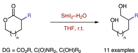
Scheme 1 The chemoselective reduction of lactones with \text{SmI}_2\text{-H}_2\text{O} enabled by the directing group effect and the rate enhancement study
