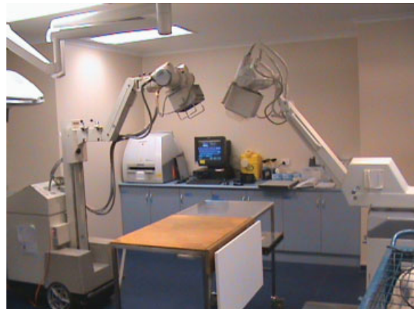
Fig. 3 The radiostereometric analysis (RSA) table used in our study. RSA setup with the roentgen tubes.
