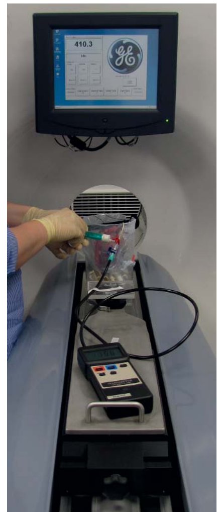
Fig. 1 Setup of the radiological investigation of a forensic sample. The hands, shown on the left of the photograph, inject the curd-contrast-agent-water mixture. A syringe, a pressure gauge (image foreground), and a catheter (image background), which goes to the vessel of the tissue sample under investigation, are connected by a three-way cock. After the injection of the contrast agent mixture, the three-way cock is closed in the direction of the tissue sample.
