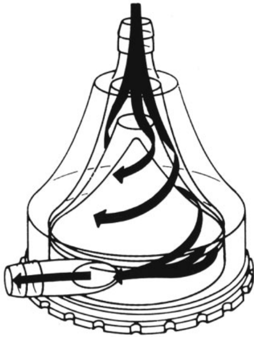
Fig. 2 Principle of a centrifugal pump; arrows demonstrate the fluid flow driven by the impeller.
