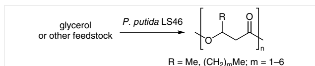
Scheme 1 The production of polyhydroxyalkanoates from glycerol or other feedstock by P. putida LS46
