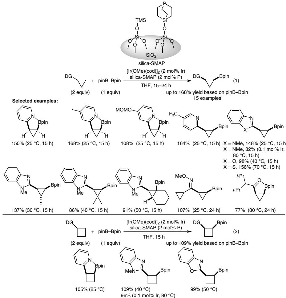
**Significance:** The heteroatom-directed C–H borylation of cyclopropanes and cyclobutanes with bis(pinacolato)diboron was carried out in the presence of  $[\text{Ir}(\text{OMe})(\text{cod})]_2$  and silica-SMAP to give the corresponding borylated products in up to 168% yield based on bis(pinacolato)diboron (eqs. 1 and 2).
