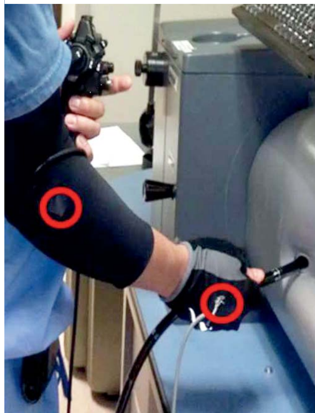
Fig. 2 Subject with magnetic position trackers held in place by custom-made arm sleeve and glove.
