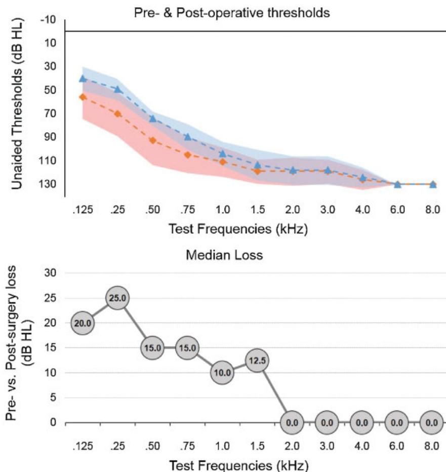
**Fig. 1** Top panel: Averaged free-field warble-tone thresholds measured pre- (blue) and post-operatively (orange) in the five patients who had successful soft-surgery with the Evo® electrode array. The shaded areas represent the standard deviation of mean. Bottom-panel: graphical representation of the median loss across frequencies for the same patients.
