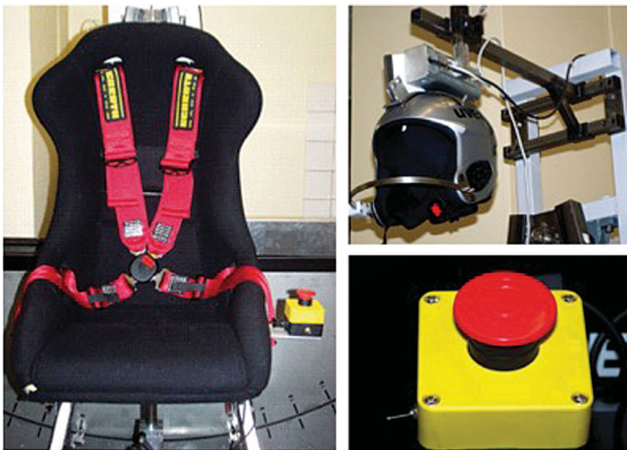
Fig. 3 Image of the 3D- trunk-excursion chair with a 4-point seat belt by Recaro (left). Enlarged Image of the so-called “emergency release button” and the magnetically fixated helmet (right). The release button enables the volunteer to terminate the experiment by releasing the magnet (right).
