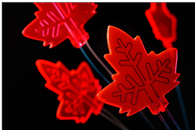
Figure 1 Luminescent solar concentrator based photomicro-reactors which allow for increased harvesting of solar light for application in organic synthetic photochemistry
