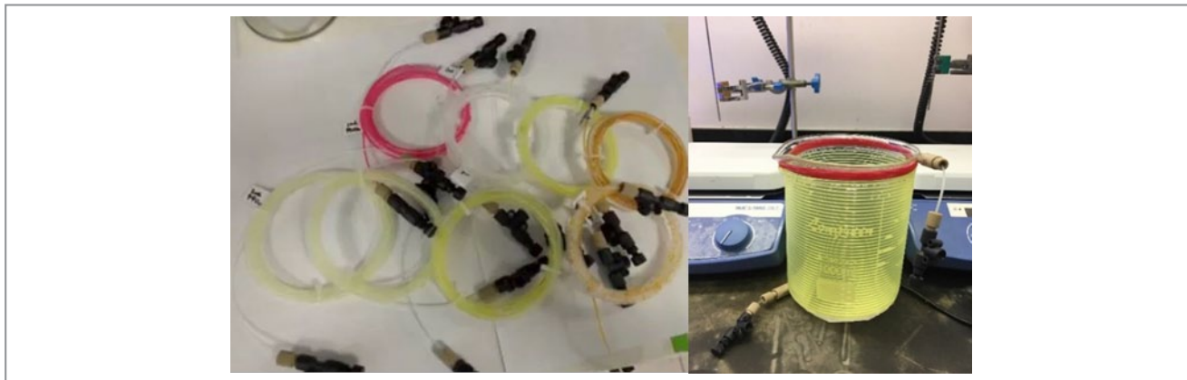
Figure 1 The “stop-flow” micro-tubing (SFMT) reactor (left: reactors for parallel screening; right: reactor with gram-scale production)
