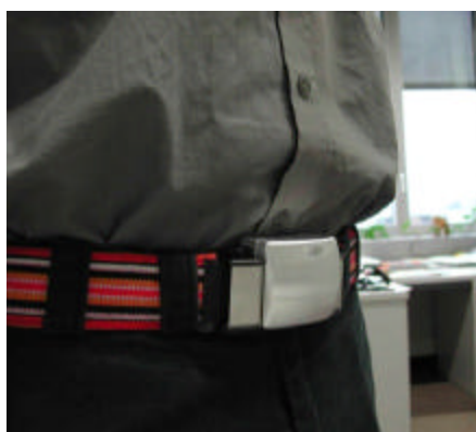
Fig. 9. ETH-QBIC – a mobile computer (Xscale CPU, 256 MB SRAM, USB, RS-232, VGA, Bluetooth) integrated in a belt buckle; the belt houses the flexible batteries and interface connectors [44].
