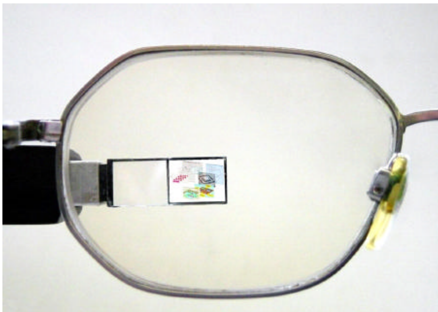
Fig. 7. Microdisplay (Microoptical Corp, http://www.microopticalcorp.com ) mounted on eyeglasses.
