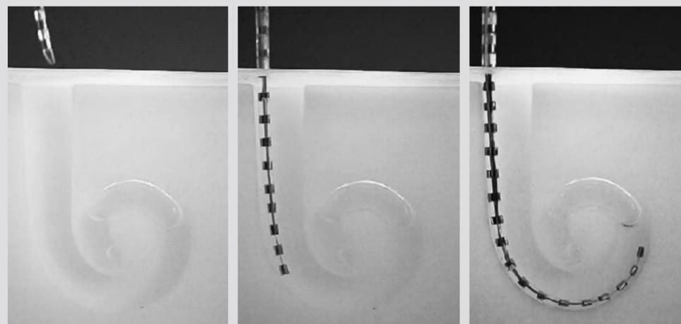
**Figure 1:** Visualization of the insertion process from the beginning (left) to the point of first contact (middle) to full insertion depth (right). At that point maximum insertion force was measured.
