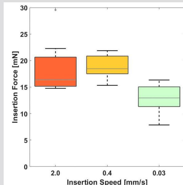
**Figure 2:** Maximum insertion forces for different speed values.
