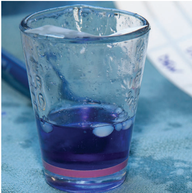
Fig. 7 Contaminated glue mixture. Polymerized glue “icebergs” indicate contamination with ionic solutions.
