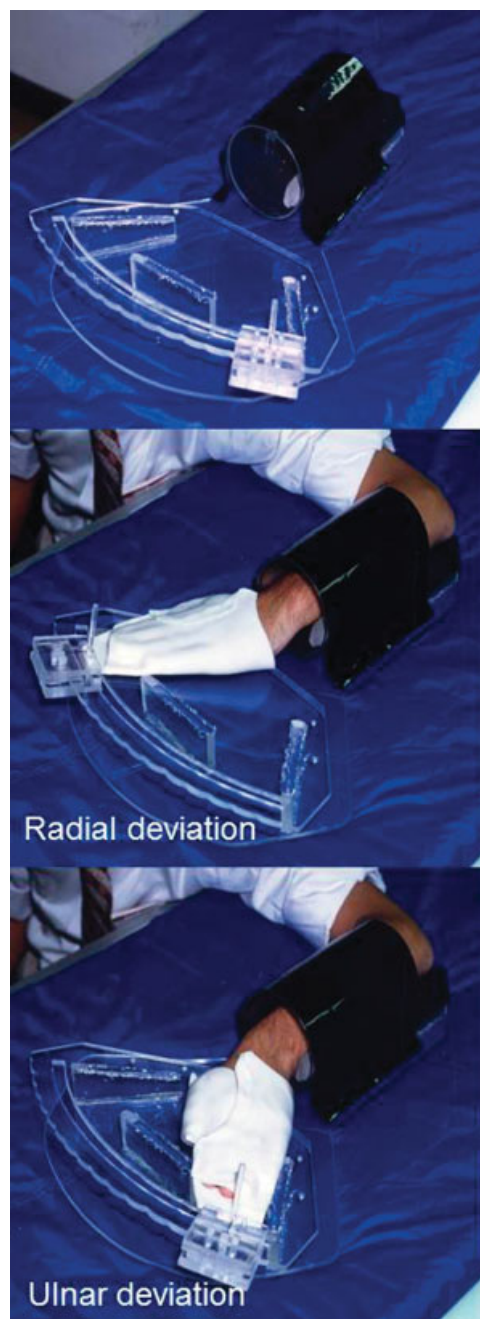
Fig. 1 All acrylic positioning device which allows 15 degrees radial deviation and 25 degrees ulnar deviation without any positional changes on flexion–extension.
