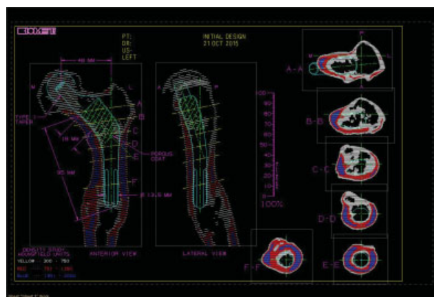
Fig. 2 Computed tomography (CT)-based blueprint of the custom prosthesis designed to accommodate the patient's proximal femoral anatomy.
