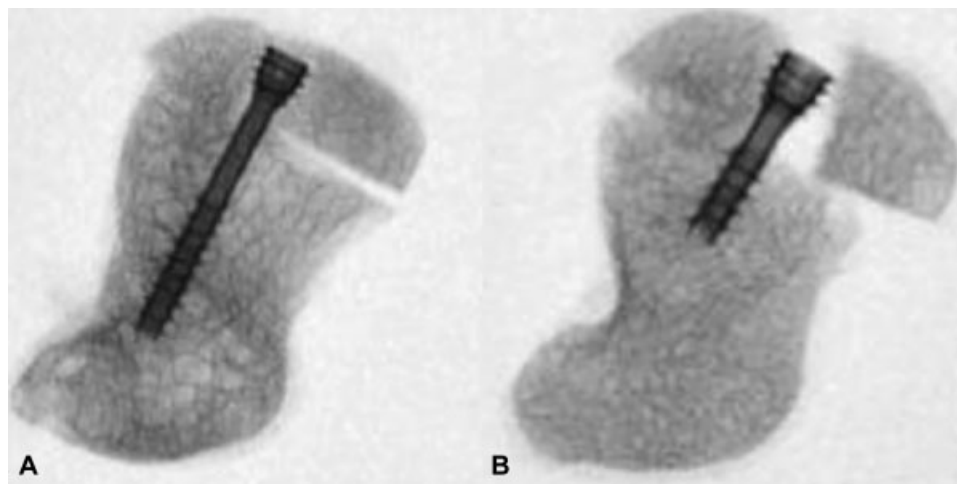
Fig. 5 Failure modes after testing with (A) failure by proximal pole fracture and (B) failure by loss of fracture reduction.
