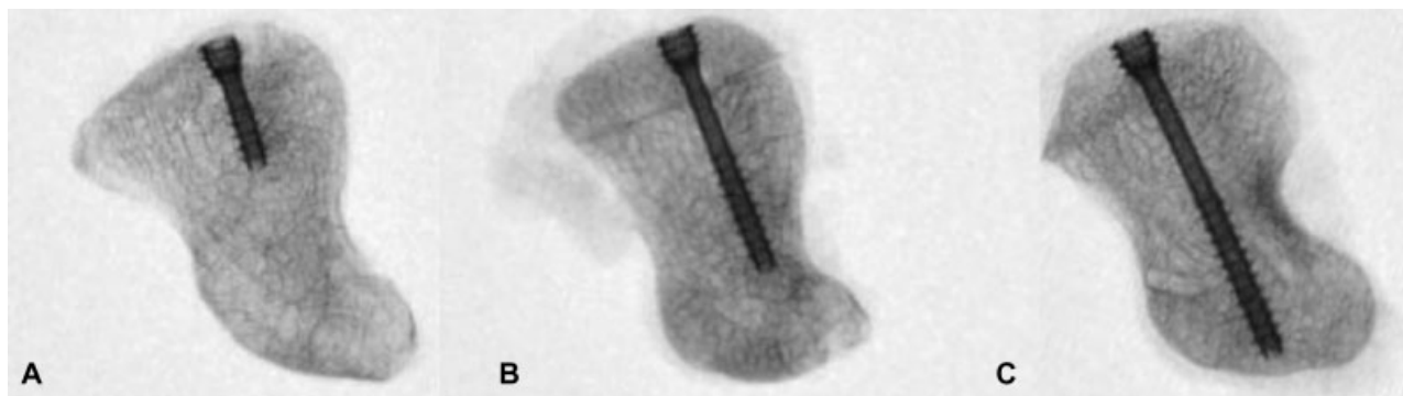
Fig. 2 Proximal 7 mm scaphoid fracture fixation construct fixed with (A) 10 mm headless compression screw (HCS), (B) 18 mm HCS, (C) 24 mm HCS.
