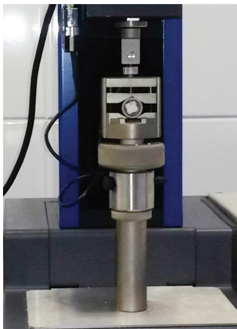
Fig. 2 Sample fixed to universal test machine.
