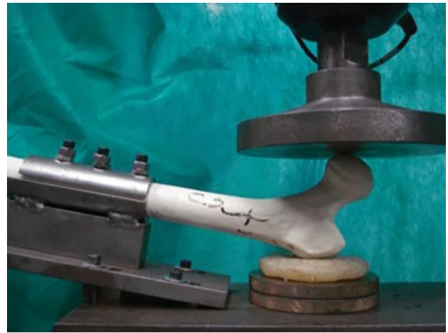
Fig. 2 Synthetic bone before the mechanical test.
