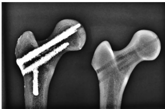
Fig. 1 Femurs radiographed after polymethylmethacrylate filling (left) and with no reinforcement (right).
