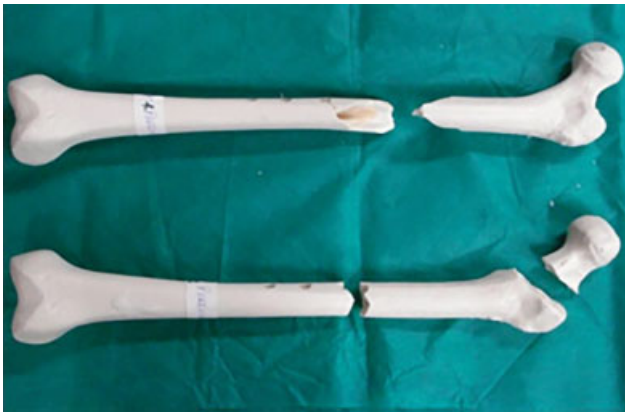
Fig. 4 Synthetic specimens with the neck and diaphysis fracture (above) and diaphysis fracture (below) after the mechanical test.
