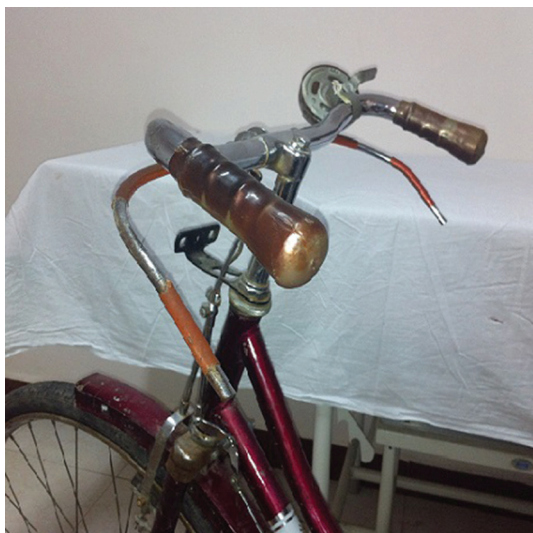
Fig. 1 The bicycle from which the child fell. The rod-like brake handle is just under 1 cm in diameter.
