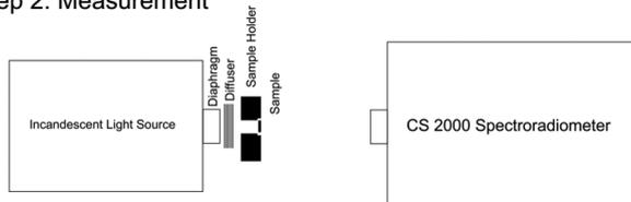
Fig. 1 Measurement of transmittance by a spectroradiometer.
