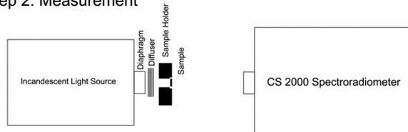
Fig. 2 Measurement of reflectance by a spectroradiometer.
