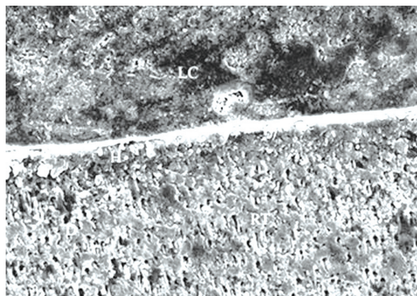
Figure 3. SEM view of demineralized specimen for Variolink II. (D:Dentin, LC:Luting Cement, RT:Resin Tags, H:Hybrid layer) (X500)
