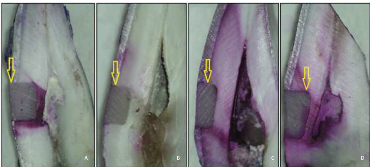
Fig. 1 The arrowheads show microleakage levels between the restoration and tooth surface of two-dimensional specimens. (A) Score 0, no leakage; (B) Score 1, leakage depth up to one-third of the internal surface; (C) Score 2, leakage depth up to two-thirds of the internal surface. (D) Score 3, leakage into more than two-thirds of the cavity depth up to the axial wall or toward the pulp.
