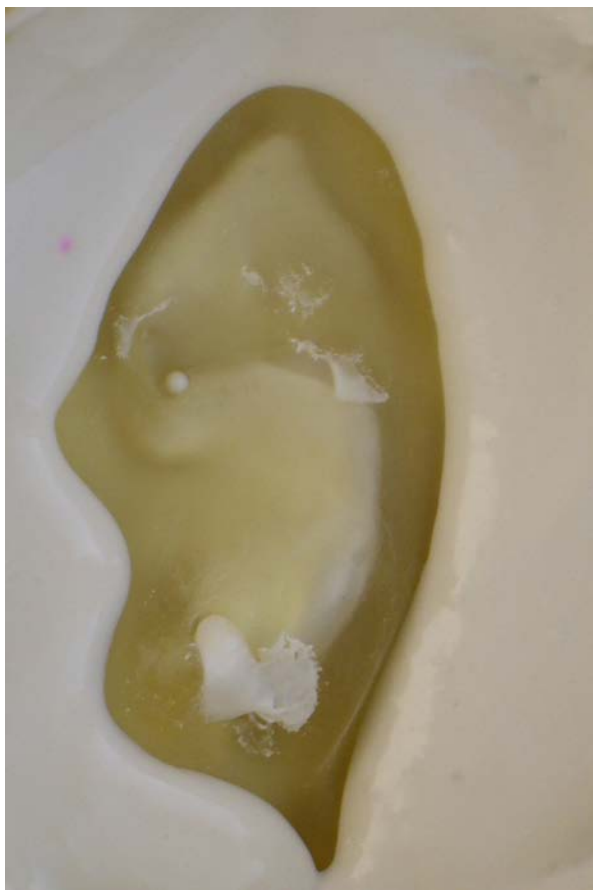
Figure 9. Stereolithographic model in the impression material.
