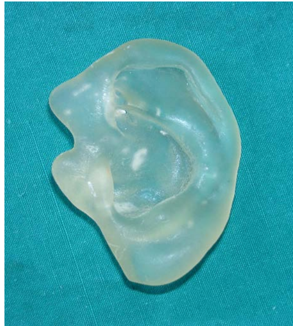
Figure 8. 3-D model obtained by stereolithography.
