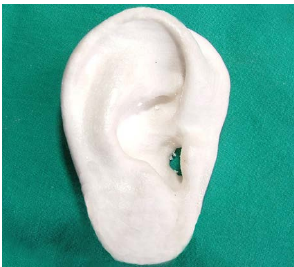
Figure 3. 3-D model obtained by 3-D ink-jet printing.
