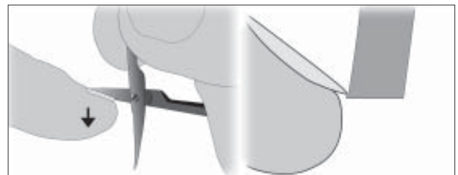
Figure 11: Sharpening scissors: feeling for the sign of completion, a “wire edge”
