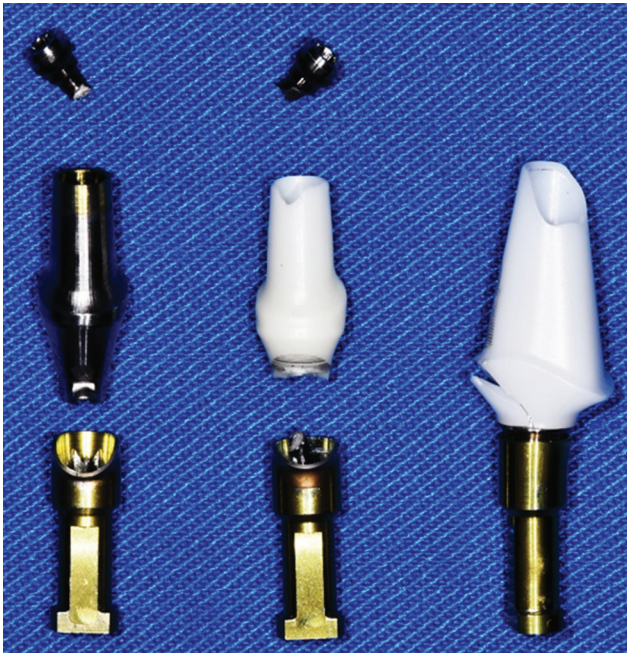
Fig. 1 An illustration of various fracture modes observed in the titanium and 1- and 2-piece zirconia abutment groups.
