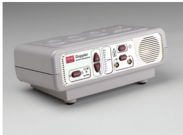
Fig. 1 Doppler blood flow monitor. Cook medical Doppler blood flow monitor. Provides primary audible and secondary visual feedback of blood flow when connected to Cook–Swartz Doppler Probe. Scale from 1 to 10—visualization of audio signal. Permission for use granted by Cook Medical, Bloomington, IN.
