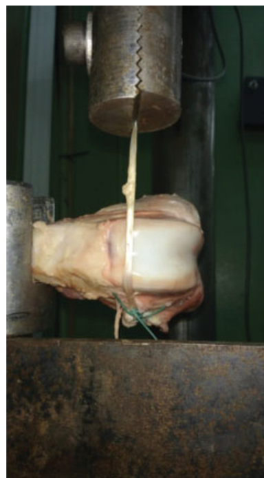
Fig. 1 Anterior view of a left porcine femur with a perpendicular graft under traction on the universal traction testing machine. Authors, 2017.
